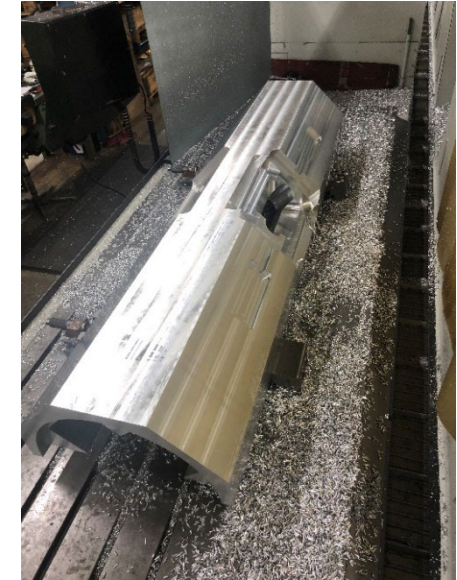
Strongback in machining, first half complete
