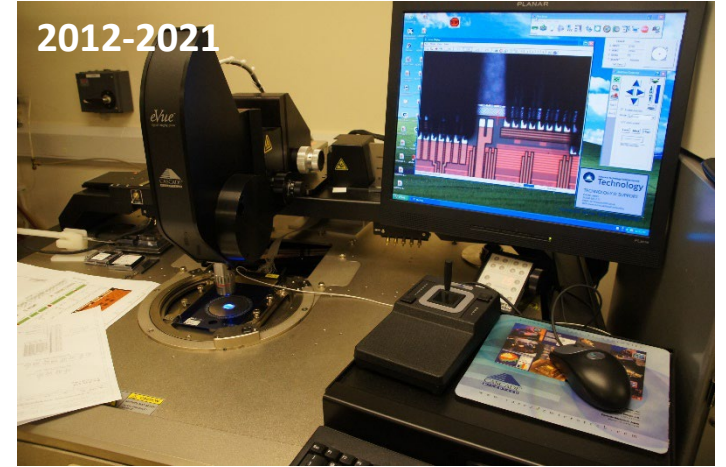
Wafer probe station testing – The ASIC is operated with all pads at full power and full images readout. Same NI systems as original chip tests.
