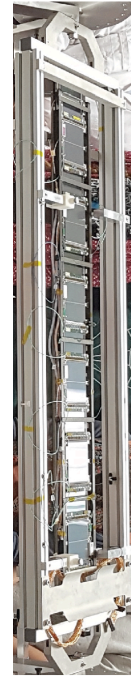
First ladder fully equipped with 12 functional modules
