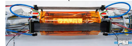
Pixel detector with 0.1 X_0 per layer, 50 \mu\text{m} HVMAPS sensors
