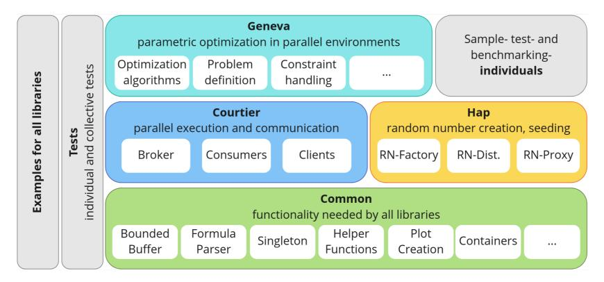
Common sublibrary: central functionality as thread pool, logger, parser, ... Geneva sublibrary: functionality specific for parametric optimisation Courtier sublibrary: template library for parallelisation Hap sublibrary: centralised generation of randomised numbers Automated unit tests, benchmarks and examples
