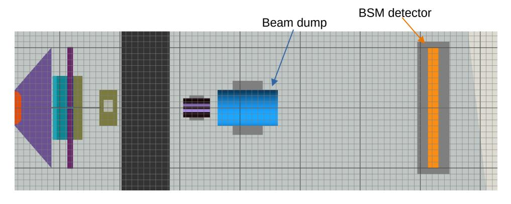
Regular geometry settings where the beam dump contains air insert
