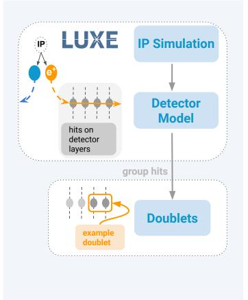
Select doublets based on the ratio  $\delta x/x_0$ where  $\delta x = x_{i+1} - x_i$ , while  $x_0$  indicates the  $x_i$  on the detector layer closest to the IP.
