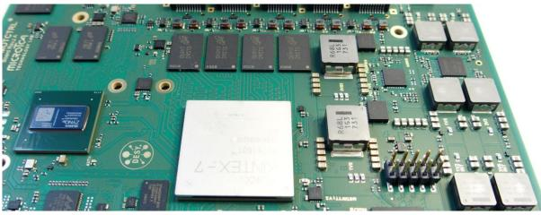
Heterogeneous approach MPSoC (2 GB DDR4) and FPGA (4 GB DDR3)
