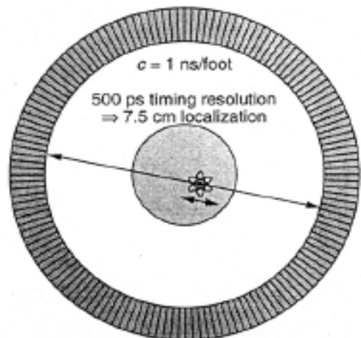
Figure 1. Time-of-Flight PET Camera. Annihilation photo detected by a ring of scintillation crystals. With a conv PET camera, this localizes the position of the positron to segment joining the two crystals. With a TOF PET cam arrival time difference is used to further restrict the positio
