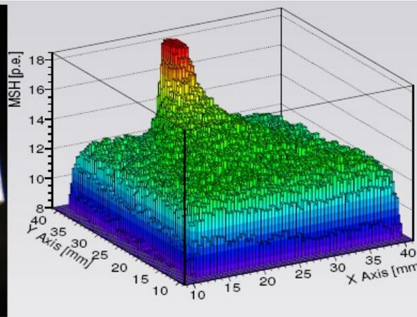
Special optimization of SiPM coupling through a dimple in the scintillator allows to recover good uniformity
