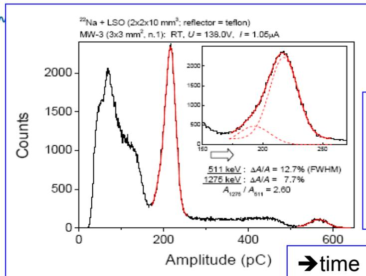
3x3mm<sup>2</sup> SiPM (Z. Sadigov) + LSO crystal (2x2x10mm<sup>3</sup>) test with <sup>22</sup>Na
