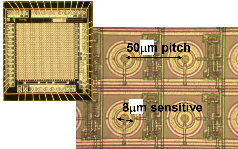
$\sim 50 \mu\text{m}$  pixel SPADs arranged in arrays
