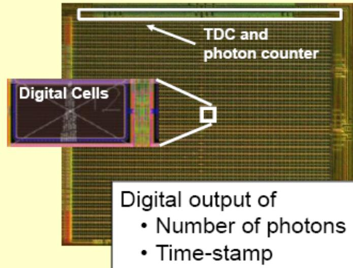
Integrated readout electronics is the key element to superior detector performance
