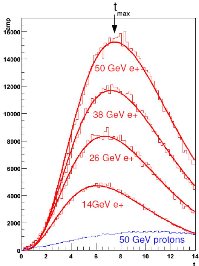
e/p separation based on different longitudinal shower shape at a given particle energy (spectrometer)
