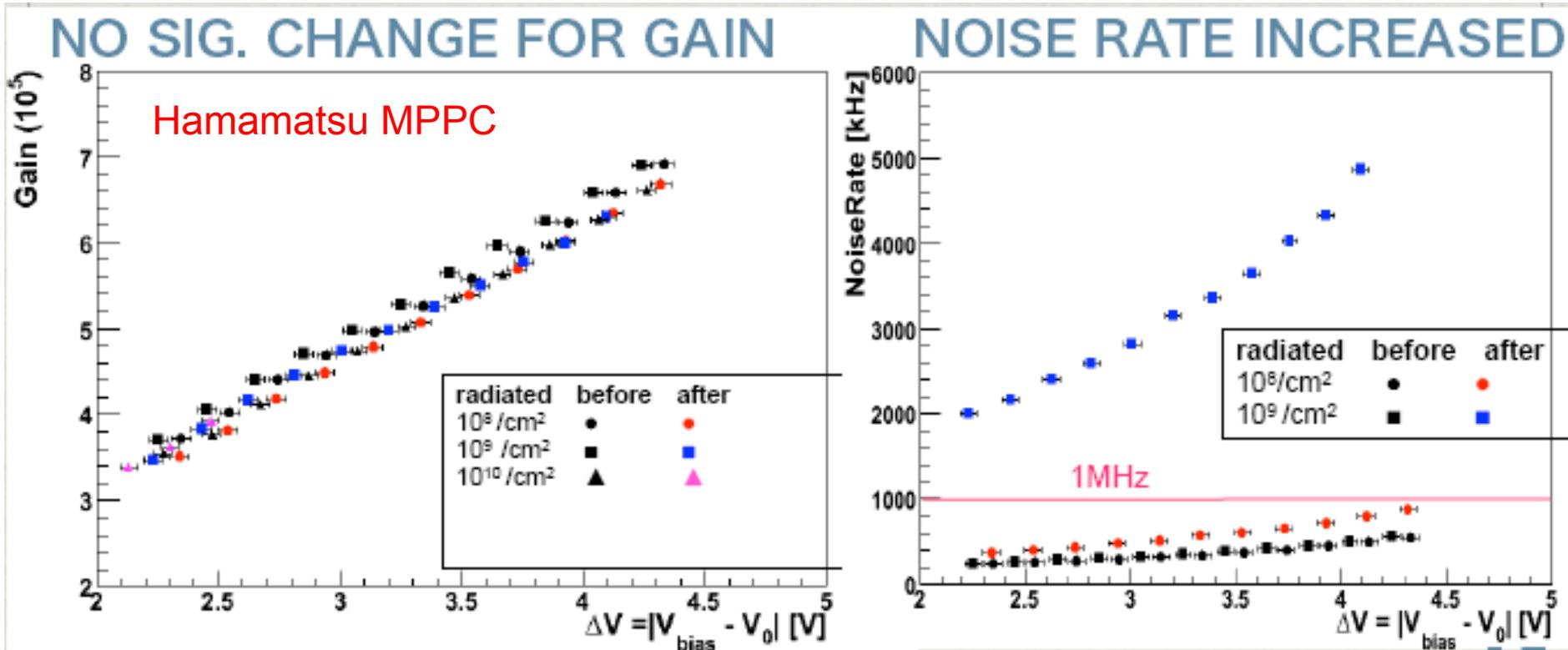
Only thermal noise increase after  $10^9 \text{ n/cm}^2$ , no other significant effects on Gain and response function
