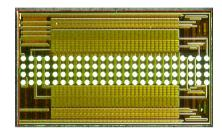
Switcher: radiation-hard switching of on-detector 20 V signals
