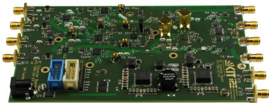
Two-stage high-frequency electronics: 800 MHz bandwidth, 4-12 GHz
