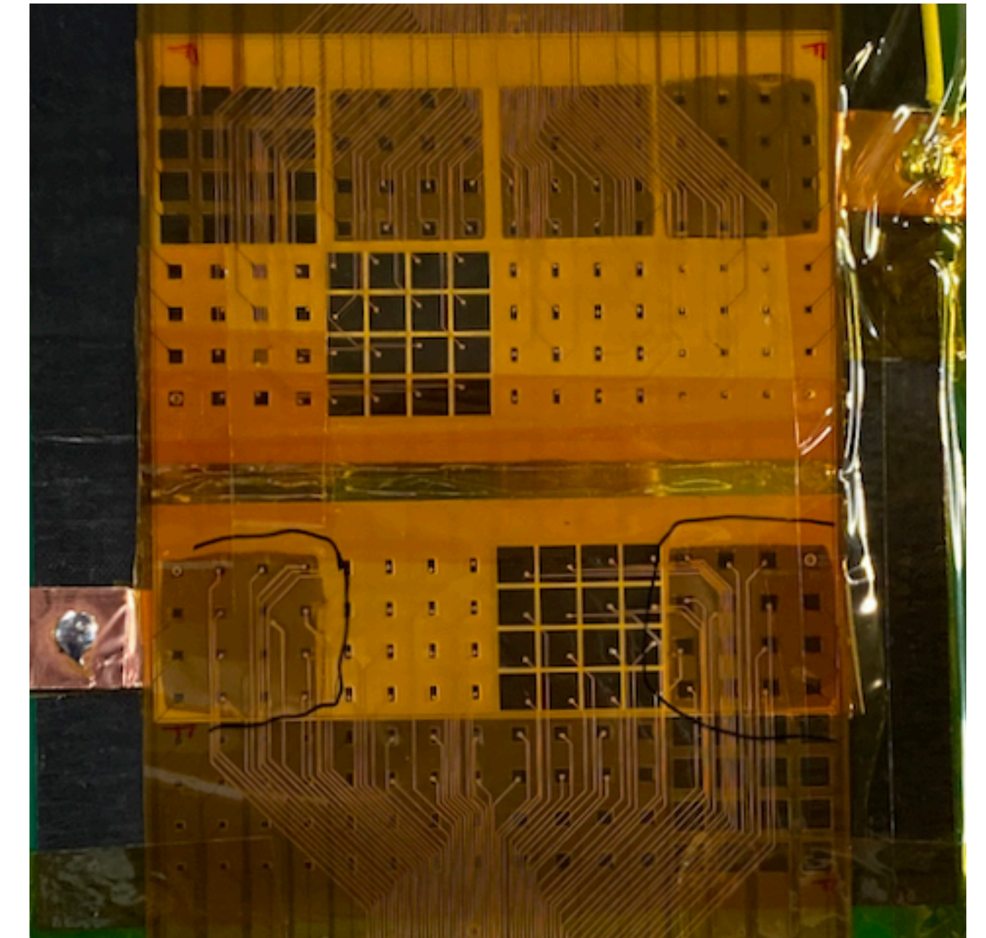
Back side of silicon sensor for test manufactured by Hamamatsu, connected with copper traces and conductive glue
