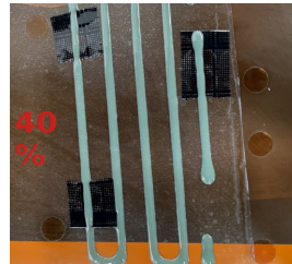
First tests with Hysol, loaded with different fractions of alumina filler
