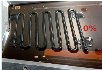
First tests with Hysol, loaded with different fractions of alumina filler
