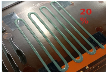
First tests with Hysol, loaded with different fractions of alumina filler
