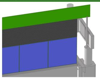
ullet Structure of PCBs (thickness: 1  $\div$  1.5 mm + chips/connectors), kapton foil and Silicon sensors
