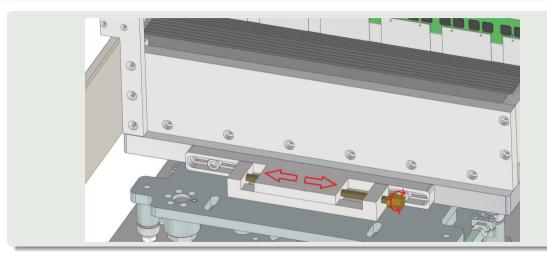
• new mechanism under design (using M12 holes for spider)... moving and docking in final position (to 1 mm gap to the shielding)
