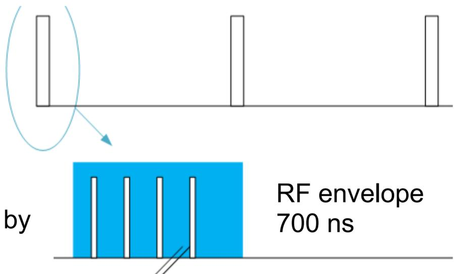
ILC/C<sup>3</sup> timing structure: Fraction of a percent duty cycle
