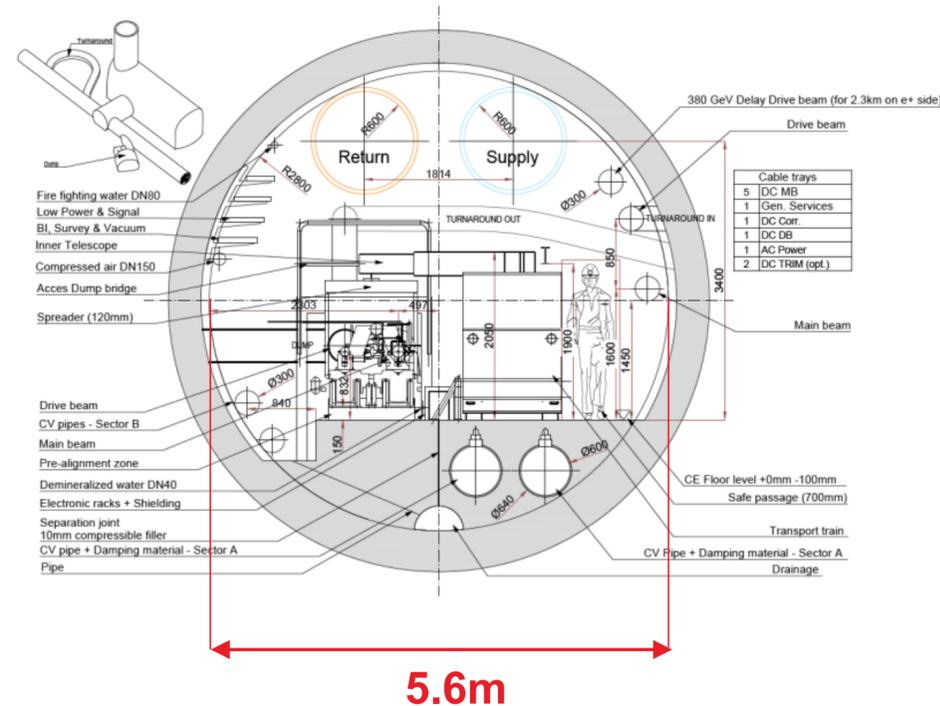
Reference: CLIC Drive Beam tunnel cross section, 2018
