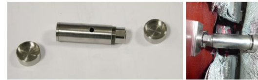
Figure 10: Outer pressure prop parts (left) and prop inserted into the cryostat (right).
