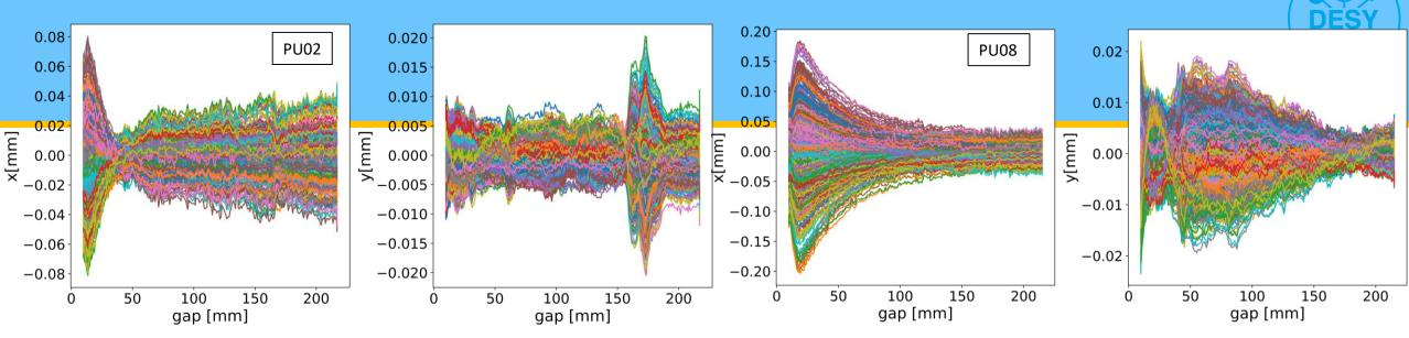
Measured orbit distortion while closing 4 undulators. Each colour represents a BPM along the ring.
