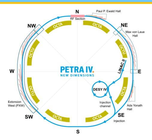
Up to **30 undulator** insertions (photon beam can be further split to allow more experimental stations).
