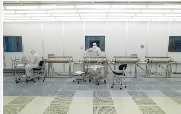
String Assembly with DESY Cavities
