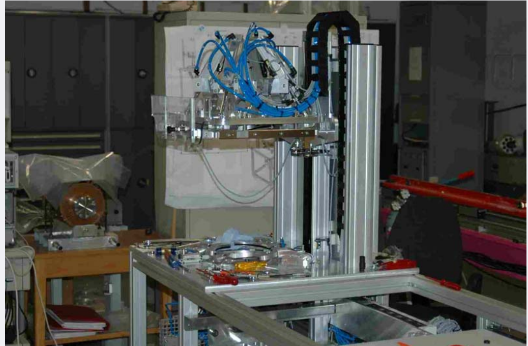
RF measurement device Equipments for RF measurement of half cells, dumb bells and end groups
