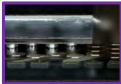
DSSC module With 8 CMOS chips Frame rate: 4.5MHz
