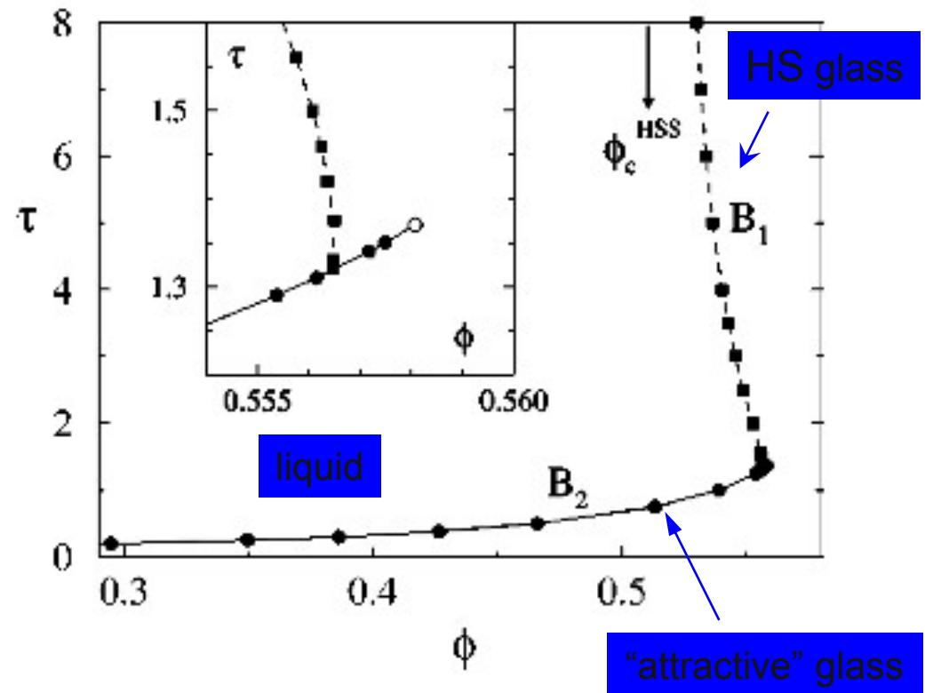
Mode coupling theory phase diagram for sticky hard spheres plotted vs. stickiness ( $\tau$ ) and volume fraction ( $\phi$ ).
