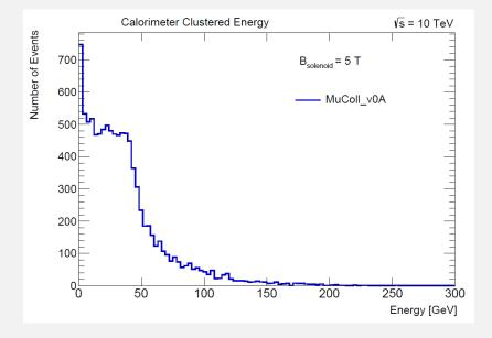
clustered energy: sum of energy of hits in the calorimeter in a cone of 0.1 radian in theta/phi around the generator level pion endpoint
