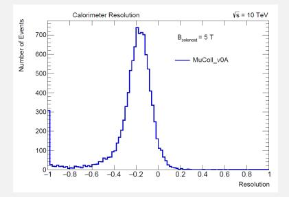
resolution plot is (clustered energy – generator energy) / generator energy
