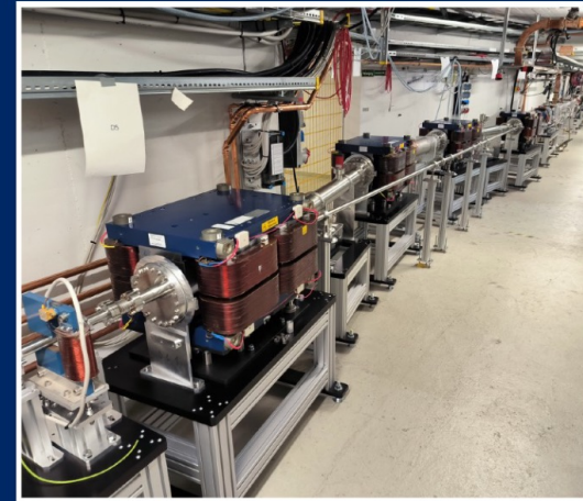
New fixed 17 cm R_{56} chicane installed
