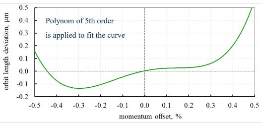
Bunch elongation is less than 0.2  $\mu$ m (0.7 fs) for particles at periphery of energy distribution  $\delta_E = \pm 0.3\% (\delta_p = 0.1\% \text{ rms})$
