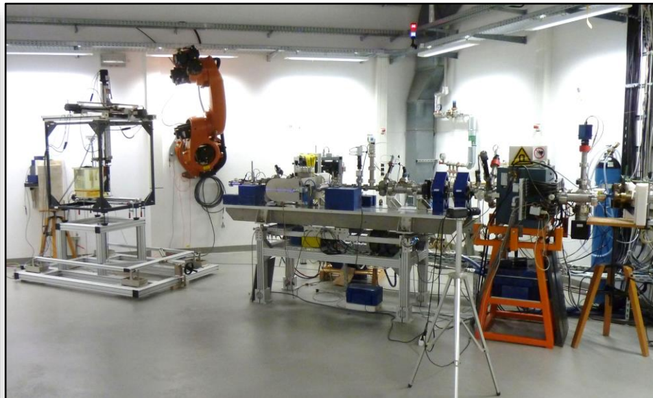
Beam line with water phantom
