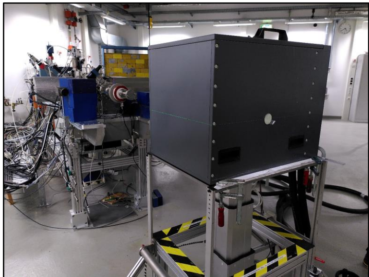
PTB's primary standard water calorimeter in ultra-high pulse dose rate electron beam
