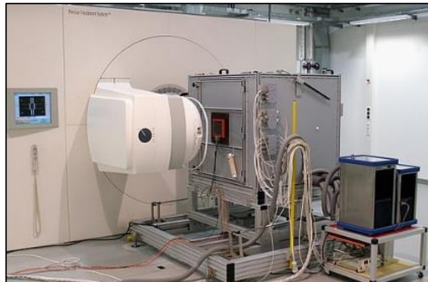
PTB's primary standard water calorimeter at a medical LINAC at PTB
