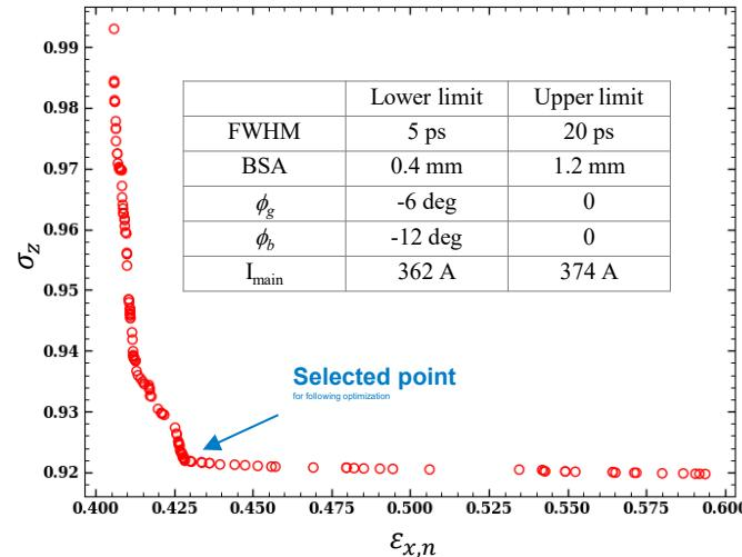
Optimized photoinjector parameters from minimizing bunch length and transversal emittance:
