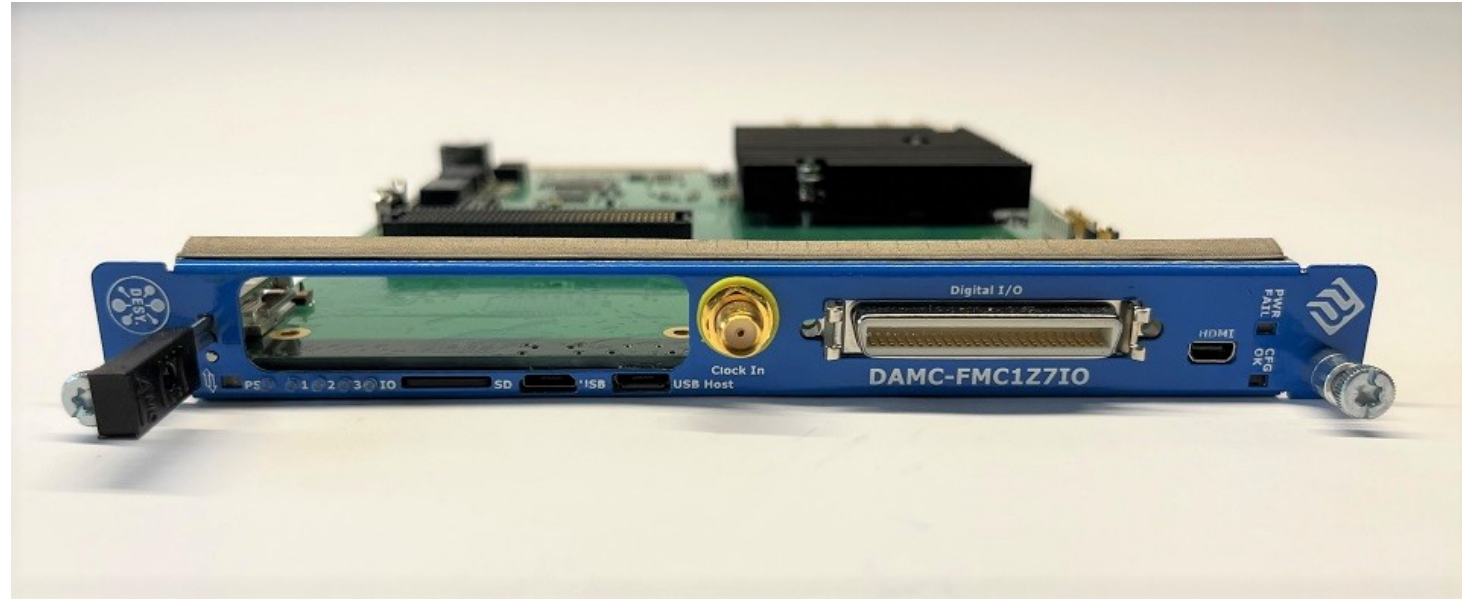
Figure: DAMC-FMC1Z7IO, fitted with a SoC from the Xilinx Zynq7000 family, from [2].
