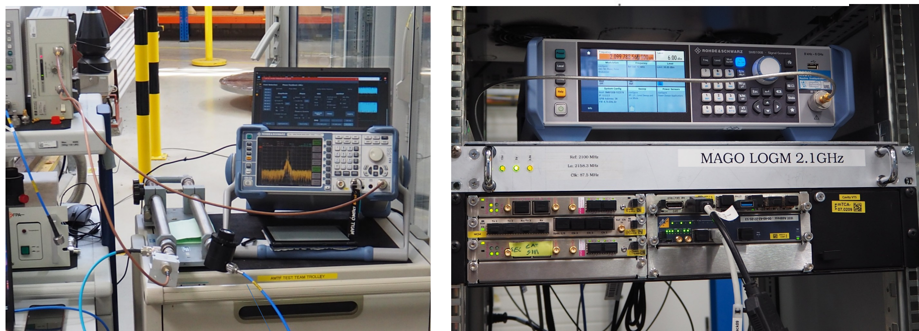
Mode rejection test setup (First 4K test of the cavity)
