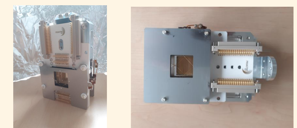
SEM Grids ready for Operation
