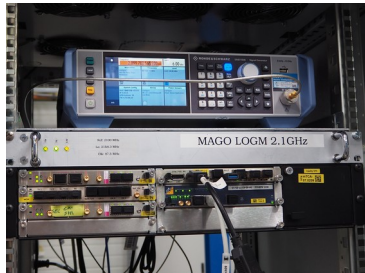
Digital self excited loop for the resonance tracking
