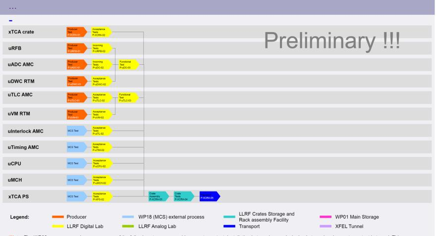
\*Note: The WP02 process map shows processes of the following stages: assembly, acceptance test, installation in tunnel, commissioning in tunnel and acceptance test in tunnel. This means that processes of the design-, development-, qualification- and purchasing stages are not included.
