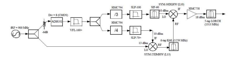
1.6 mdeg (3.4fs) [10 Hz - 1 MHz]<sub>-12t</sub> (simulation shows the same value)
