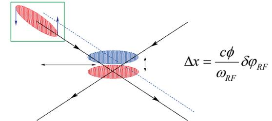
Fig – Phase offset leading to transverse displacement on one beam only [16]
