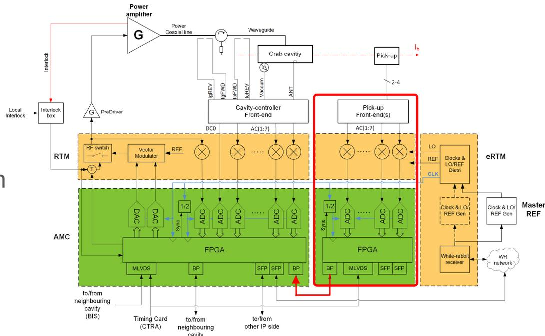
Fig – HL-LHC Beam phase & tilt measurement, alternative with dedicated AMC+RTM
