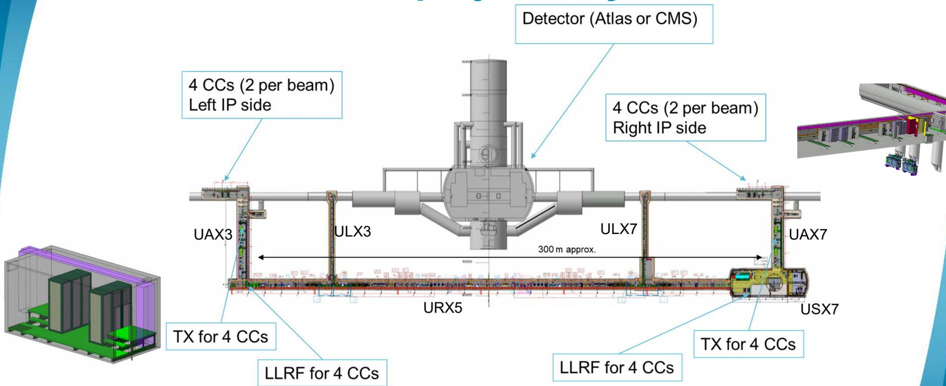
Fig – HL-LHC point 1 or 5 underground layout [1] . Top view
