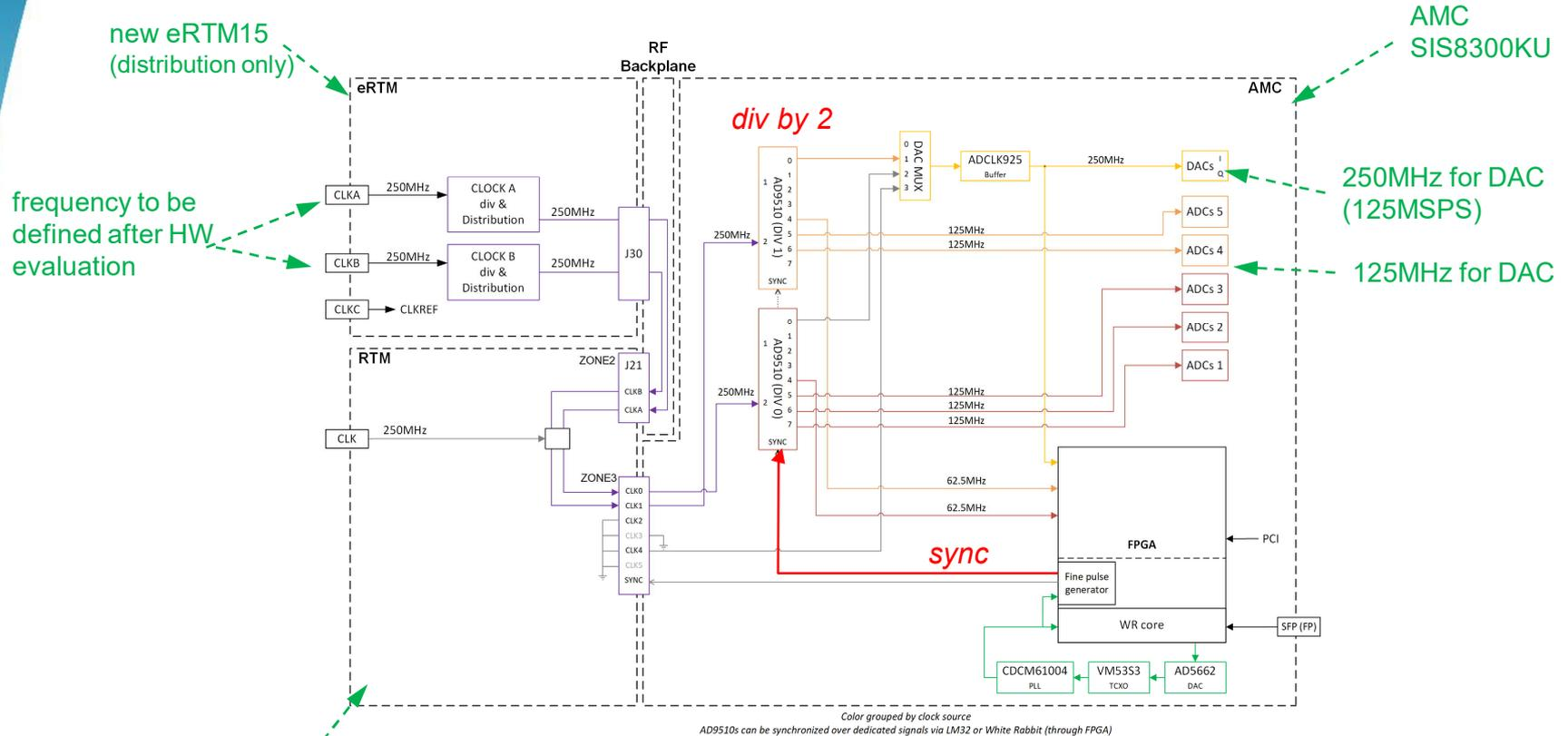
Fig – Clock distribution from eRTM to ADC& DAC on SIS8300KU
