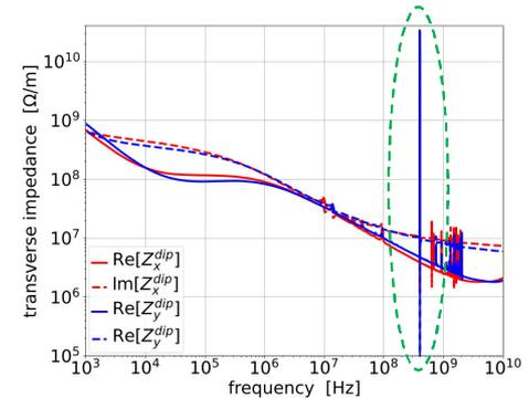
Fig – HL-LHC transverse impedance including crab-cavities fundamental mode [5] .
