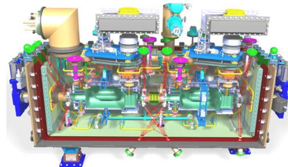
Fig – RFD Cavity and cryomodule (horizontal crabbing)
