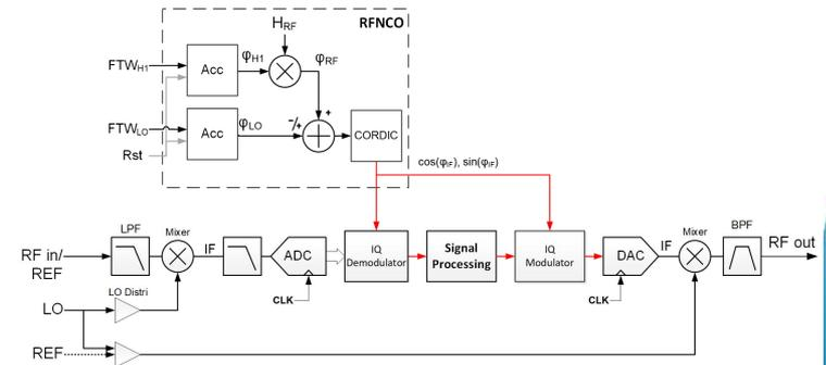
Fig – RF up/down modulation scheme
