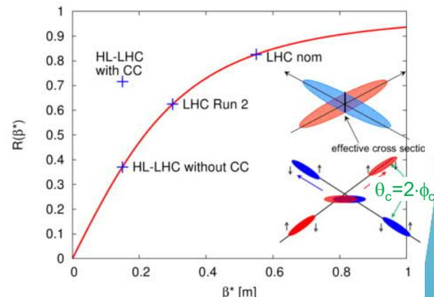
Fig – Variation of the geometrical luminosity reduction factor with  $\beta^*$  [4]
