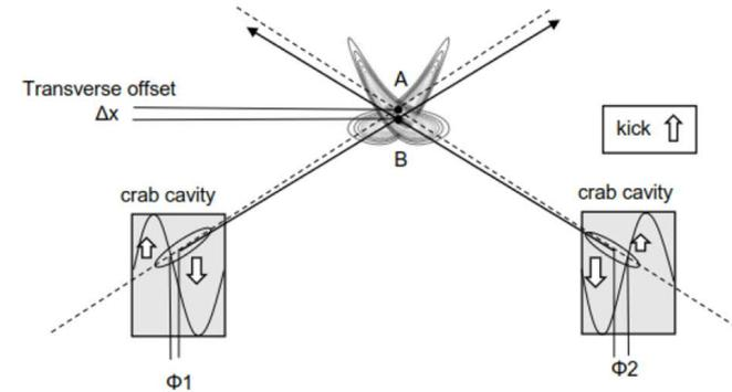
Fig – Identical phase shift for colliding bunches  $\phi_1=\phi_2$
