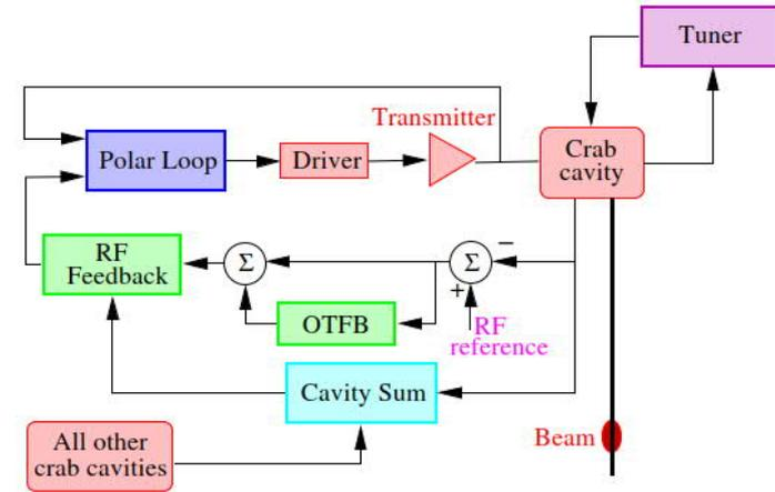
Fig – Crab Cavity Low-Level RF block diagram [11]
