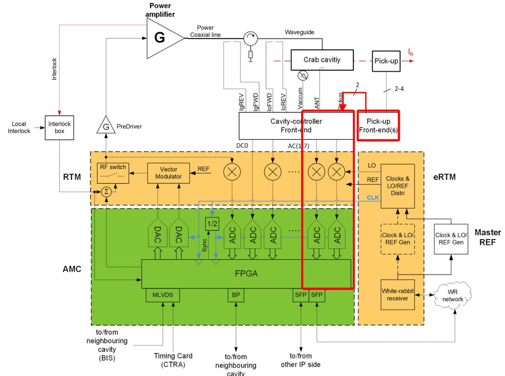
Fig – HL-LHC Beam phase & tilt measurement, alternative with dedicated AMC+RTM
