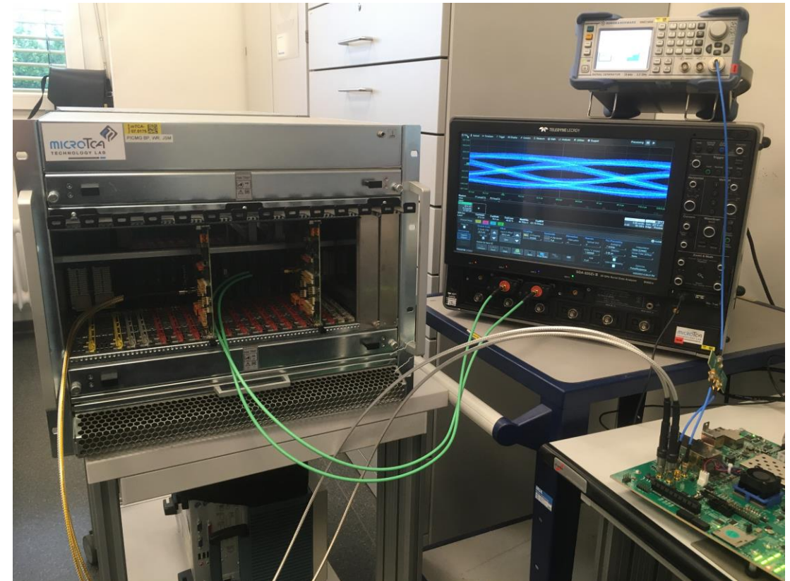
Test Setup: 10Gbps Signal Generation with IBERT on ZCU102
