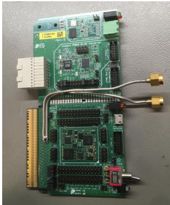
Soldered-in semi-rigid cables for reference measurement (Harting/ITB/Rompa)
