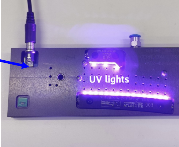
cured using UV-light
