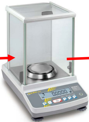
100 resin : 9 hardener (measured with a scale)
