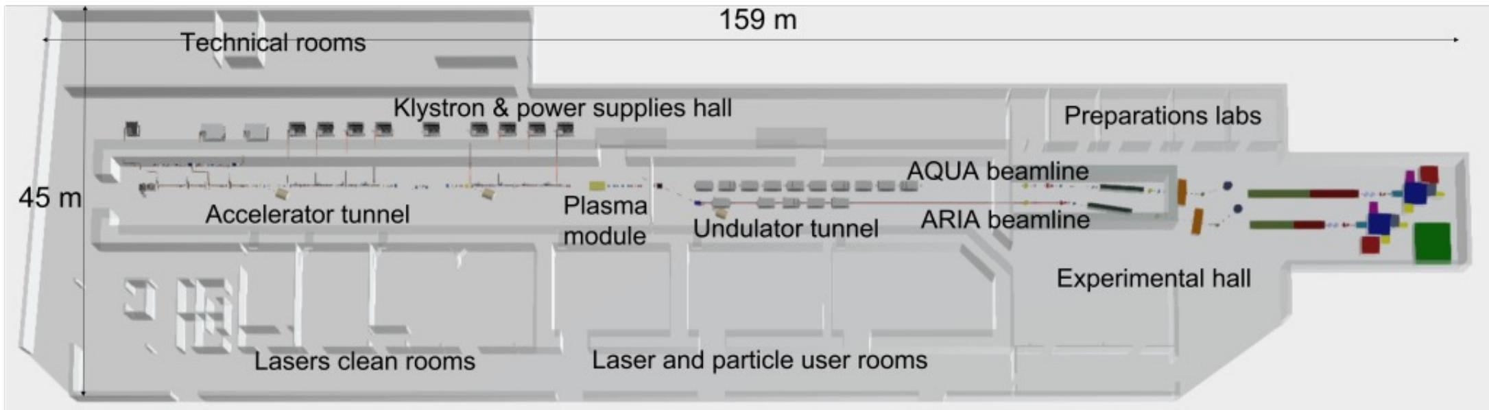
EuPRAXIA (European Strategy Forum on Research Infrastructures (ESFRI) Roadmap of 2021): a compact FEL source, equipped with user beamline at 4 nm wavelength, driven by a high gradient plasma accelerator.
