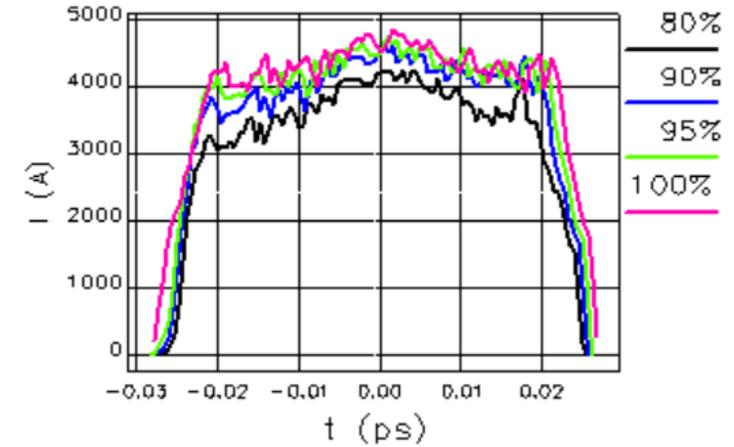
Longitudinal distribution of the electron beam current (above) and of its transverse phase space emittance (below) at the 6 GeV linac exit
