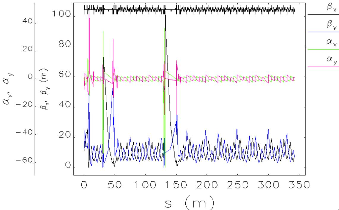
Twiss function along the C-band booster linac
