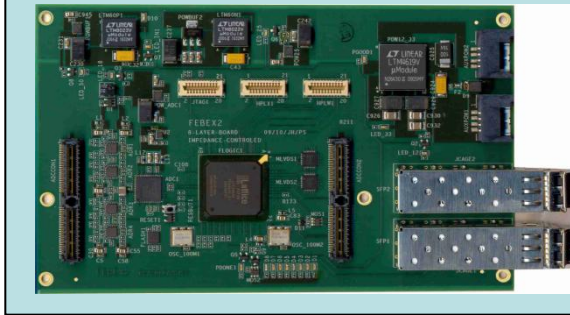
FEBEX2 - 8 channel pipeline ADC Front End Board
