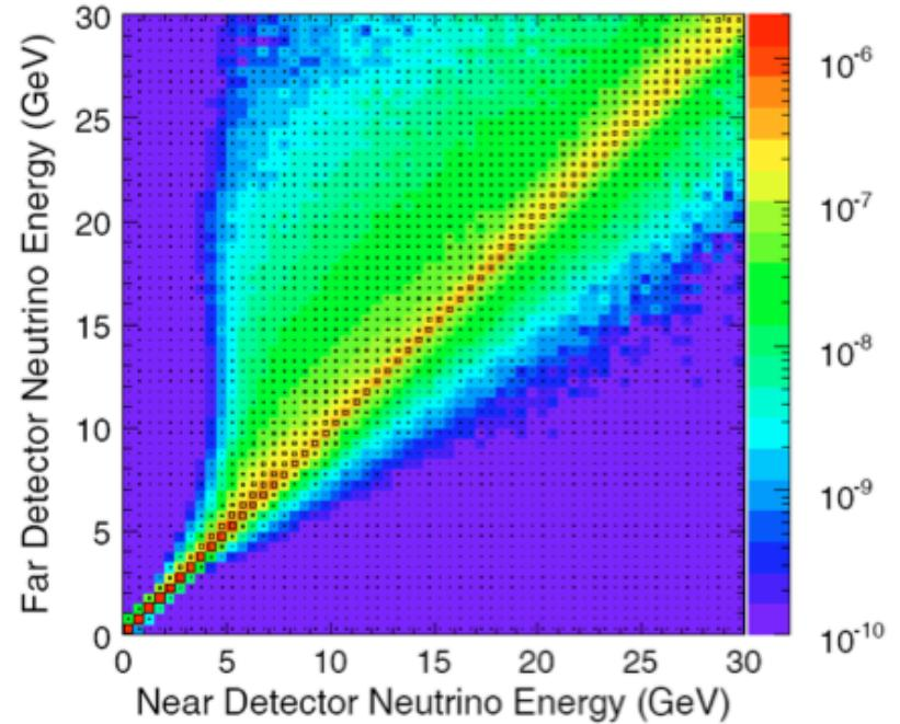
Near Detector energy spectrum extrapolated to Far Detector, using MC to provide energy smearing and correct for detector acceptance
