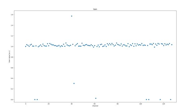
O By comparing the gain measurement from the entire injection board with a single injector, differences were obtained between the channels on the injection board
