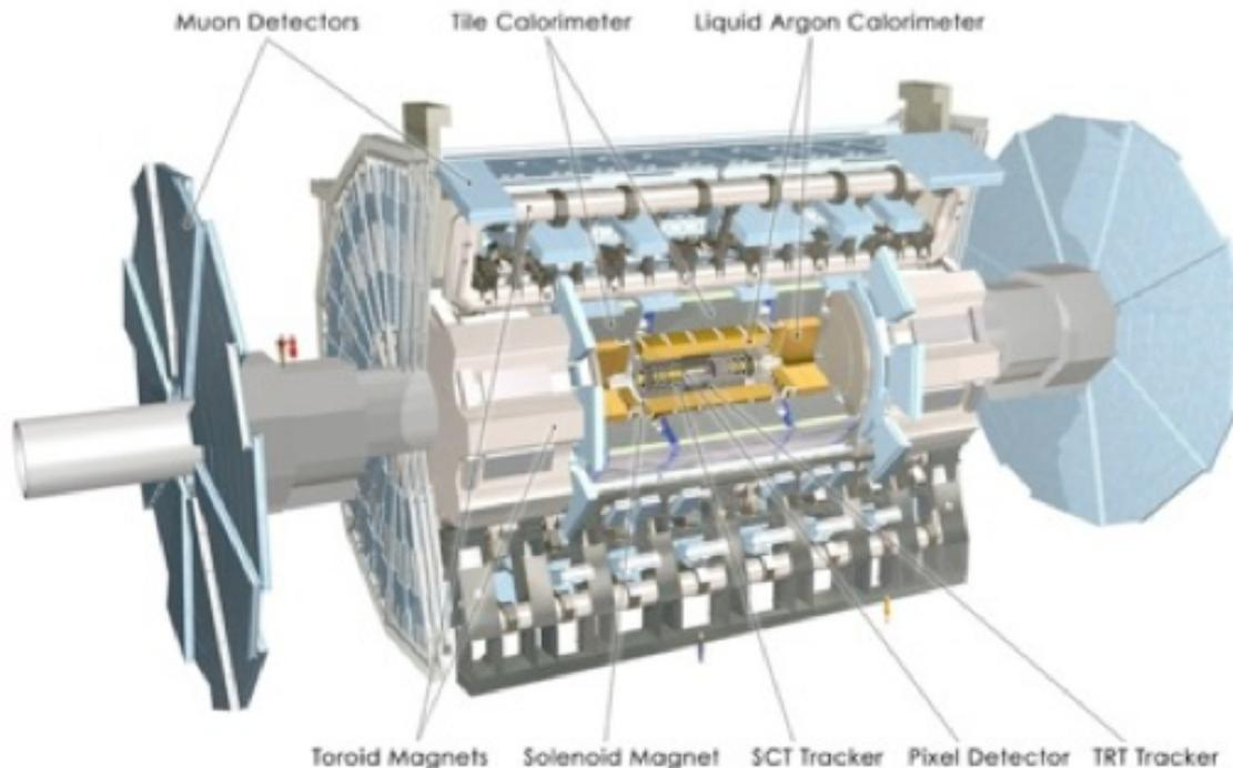
→ **The design of ATLAS was partially driven to provide high sensitivity to Higgs production**
