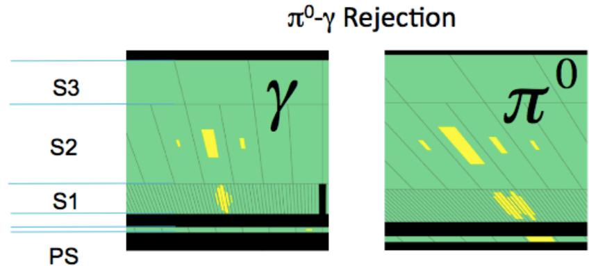
→ Converted photons have different showers from unconverted photons
