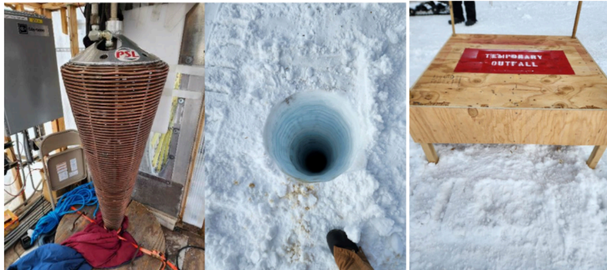
Figure 3 (left) IFD carrot, (center) hole in the firn, (right) cover for the temporary outfall (Photos: K. Studt/PSL).
