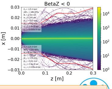
γγ interactions are independent of the e<sup>+</sup>e<sup>-</sup> process, but can happen simultaneously to it (overlay-on-physics events ) or not (overlay-only events)
