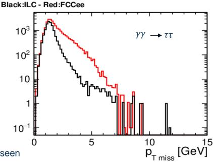
Dramatic effect in the  $\mu\mu$  case, where all the  $p_T$  of the pair is seen Cut in  $p_{Tmiss}$  10 times higher for getting the same rejection
