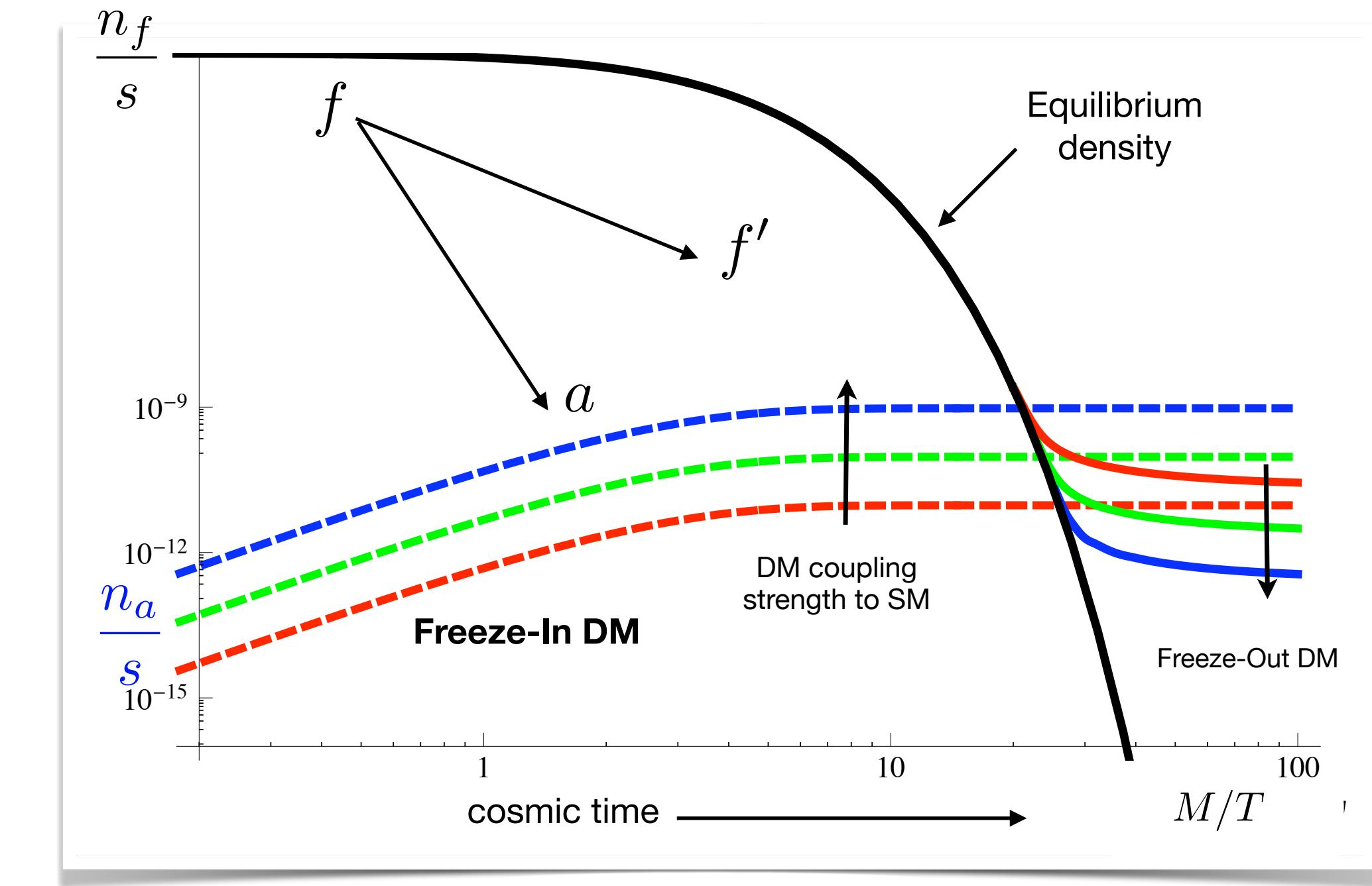
for decay of SM particle  $f$  with mass  $M$
