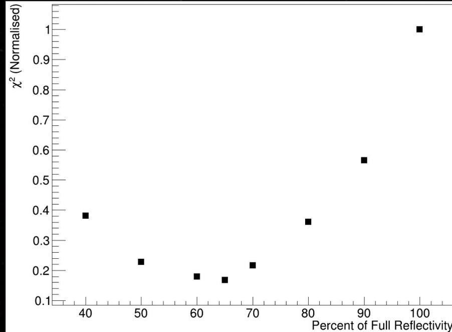
Comparison of data with simulation at 65% reflectivity shows a close match
