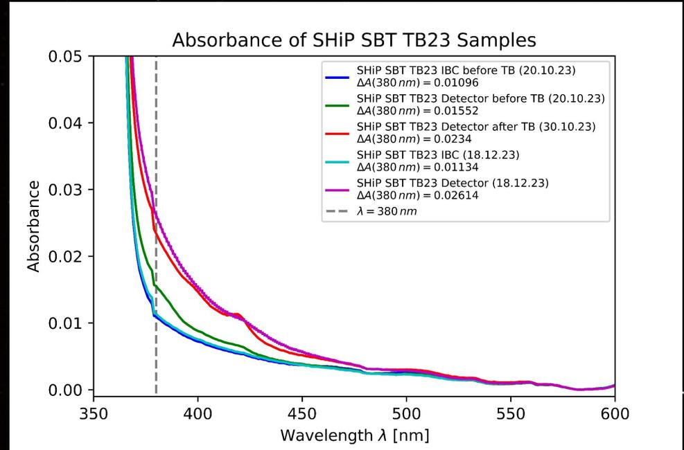
Absorbance spectra of TB 2023 taken from IBC and detector at different times
