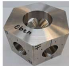
Various sample holders so that solid samples and foils can be polished
