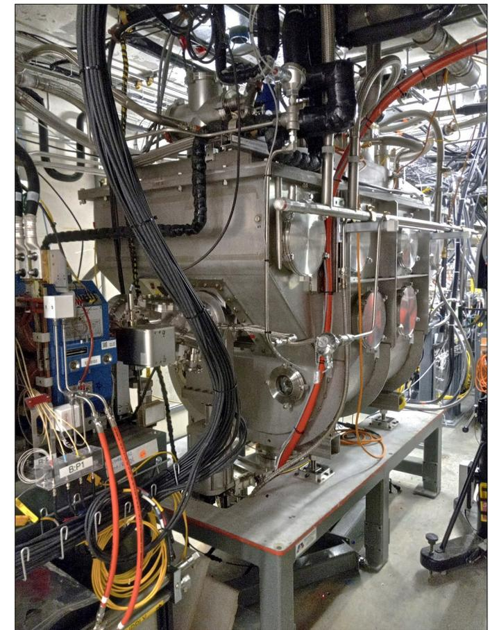
BLS Cryomodule installed and cooled down
