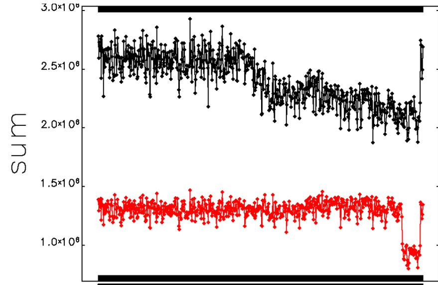
BPM sum signal over 1 turn showing beam loss during beam dump: distributed beam loss without collimator (black) and localized beam loss with collimator inserted (red). Turn 98 after beam dump command is shown
