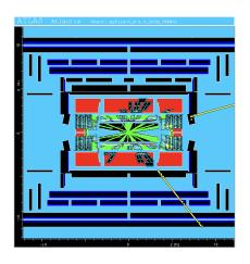
This event from Standard Model ttbar production also has high  $\,p_{\rm T}\,$  jets and muons, and some missing transverse energy.
