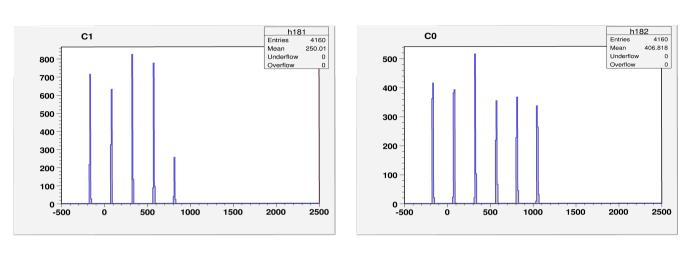
Pixel address in 5 signals: C1,C0 d-columns 0..25 A2, A1, A0 rows 0..79 each with 6 analog levels. All well separated. Decode  $\rightarrow$  col, row.
