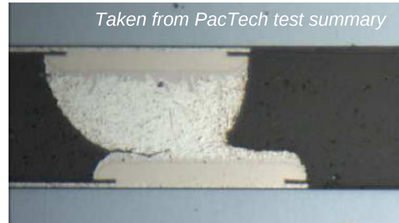
Cross sectional view after tacking
