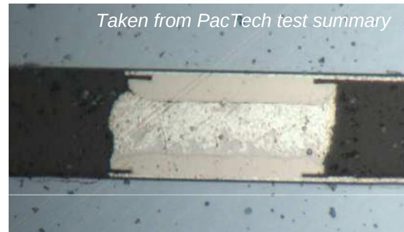
Cross sectional view after reflow
