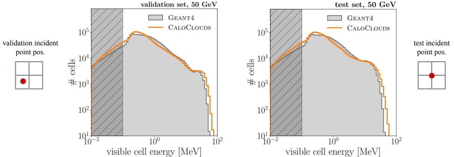
Per-cell energy distribution for the 50 GeV validation (left) data set, created at the same position as the training data set and for a 50 GeV test (right) data set simulated at a different position with the generated point cloud translated to this position
