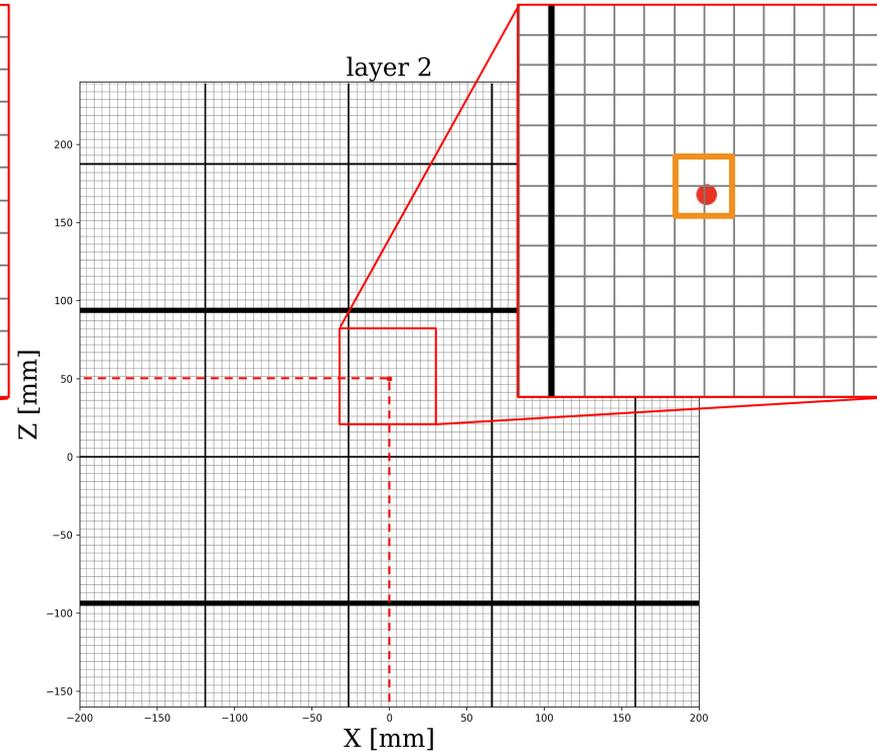
White squares represent **active cells**. Black lines are wafers, construction gaps, etc. (**not active material**)
