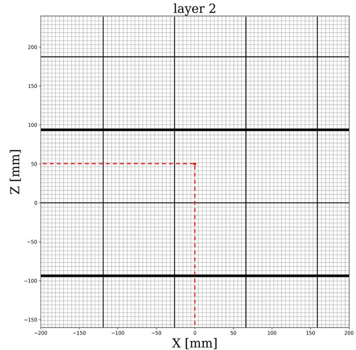
White squares represent **active cells**. Black lines are wafers, construction gaps, etc. (**not active material**)
